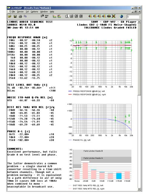
Figure 1 A Typical Results Sheet for a good CD Player
