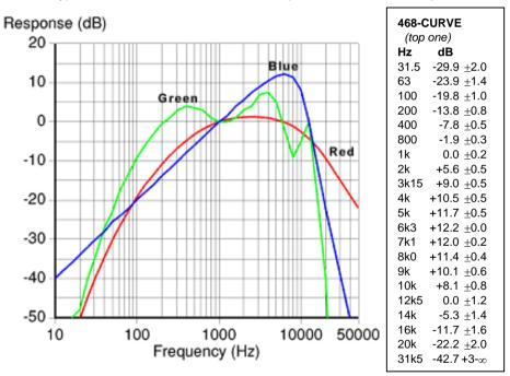
telephone line clicks. The result was a combination of frequency weighting curve and quasi-peak rectifier close to what we now call 468-Weighting.
