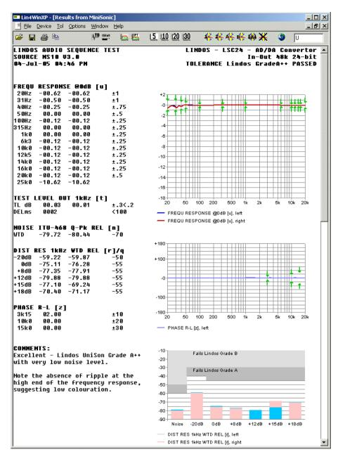
Fig 2 A Typical Results Sheet for a good 24-bit Digital Convertor
