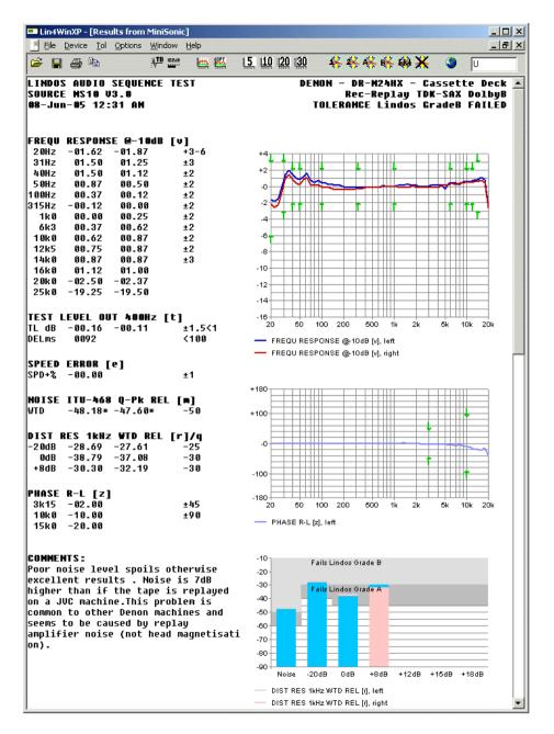
Fig 3 A Typical Results Sheet from a Compact Cassette Machine
