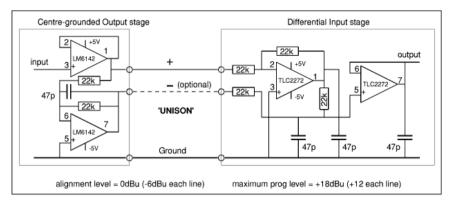
UniSon Input and Output circuits as implemented on the MS10
